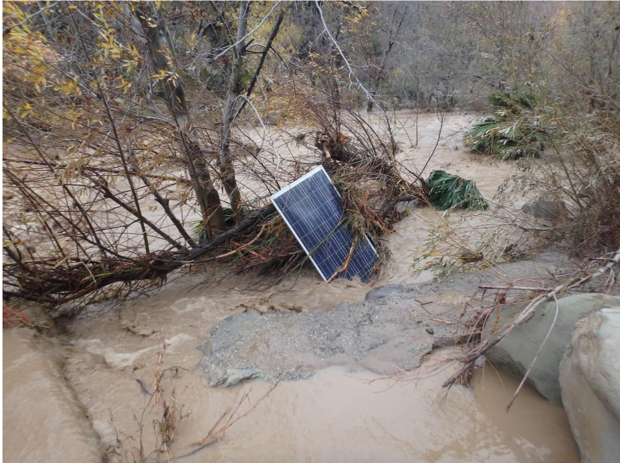
Figure 13. Damage to the North Fork Matilija Creek (NFM) stationary PIT array caused by high flows. The final of three winter storms over the course of one week in January 2019 caused the Ventura River to exceed 13,500 cfs. The associated debris flows damaged array equipment at both deployment sites, including the solar panel, pictured here. Image was taken on January 17, 2019 facing upstream.
