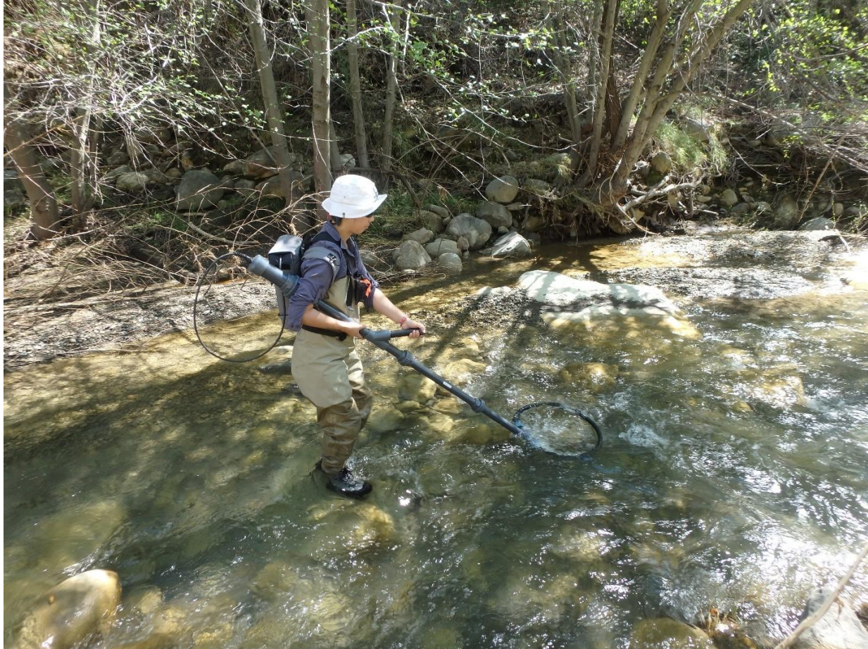
Figure 3. Image of PIT scanning survey in Upper North Fork Matilija Creek in March 2017. PSMFC Fisheries Biologist Jean Tsai operates a portable passive integrated transponder (PIT) detection device to scan all wetted habitat while progressing upstream. Following HDX PIT tagging surveys, tag scanning surveys were performed every month or when conditions allowed.
