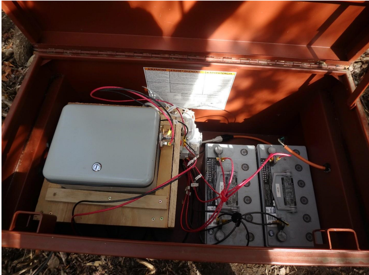
Figure 5. Image of the Ventura River mainstem (VEN) stationary PIT array design. Due to an agreement with Ojai Valley Sanitation District the Ventura River array was provided AC power. An extension cord plugged into a GCFI outlet runs to a metal jobox where it is connected to a relay is wired to the battery charger, timer, PIT tag reader, and two 12-volt batteries. The relay ensures battery charging is isolated from powering of the reader and reduces any electrical noise interference.
