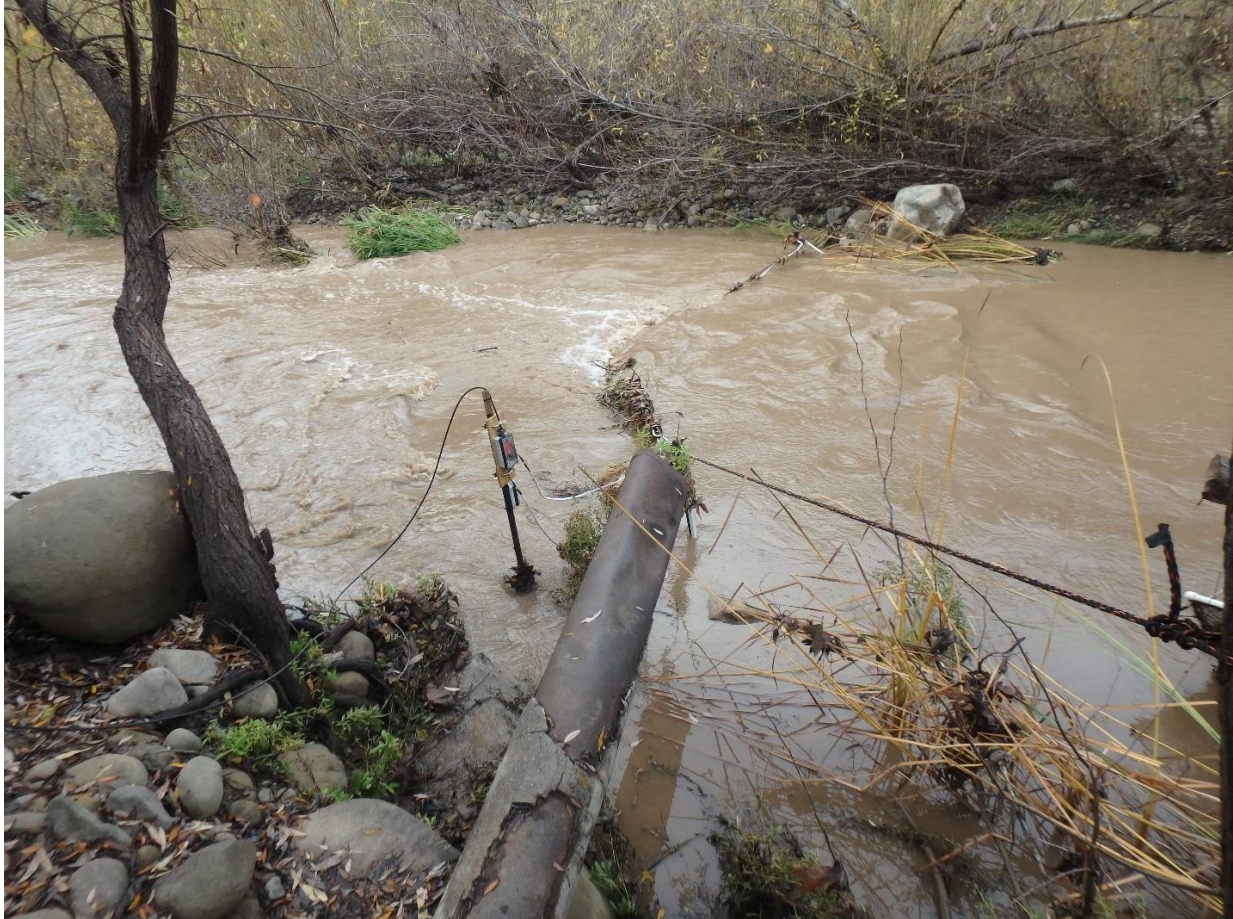
Figure 11. Image of the Ventura River (VEN) stationary PIT array in high flow. The VEN array pass-through antenna entangled in vegetation and woody debris as flows react to a storm in January 2019. The tuner box is pictured mounted on a metal T-post secured in the streambed on river-left. Image was taken facing downstream towards river-right.
